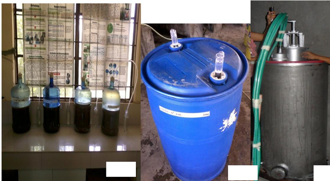
Fig. 1. Fermentation set up at laboratory (a) and Upscale condition (b) and (c)
