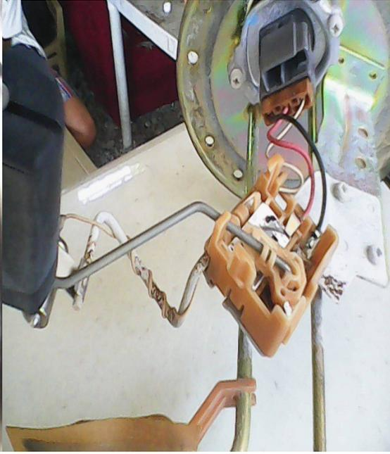
Fig 6. Floater with sign of rust formations
