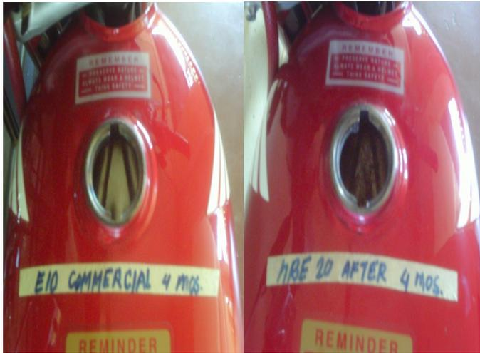
Fig 8. Rusting in the Fuel tank of TMX using hBE 20
