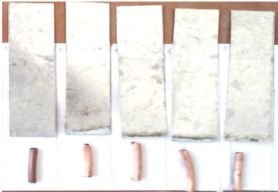
Figure 13. Rust Test in GI sheet and copper tube materials
