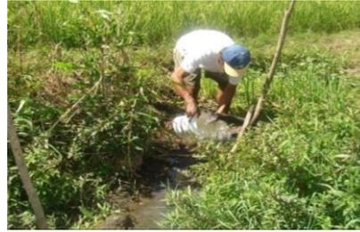
**Fig 1** Determining flow of supply by running water into a bucket of known volume.
